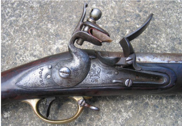
From c1759 Marine and Militia Pattern Brown Bess with goose neck cock From c1796 BM India Pattern Brown Bess with ring neck reinforced cock
