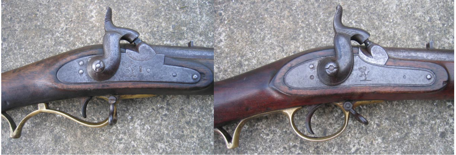
c1833? BEIC flintlock musket converted to percussion from c1837?
